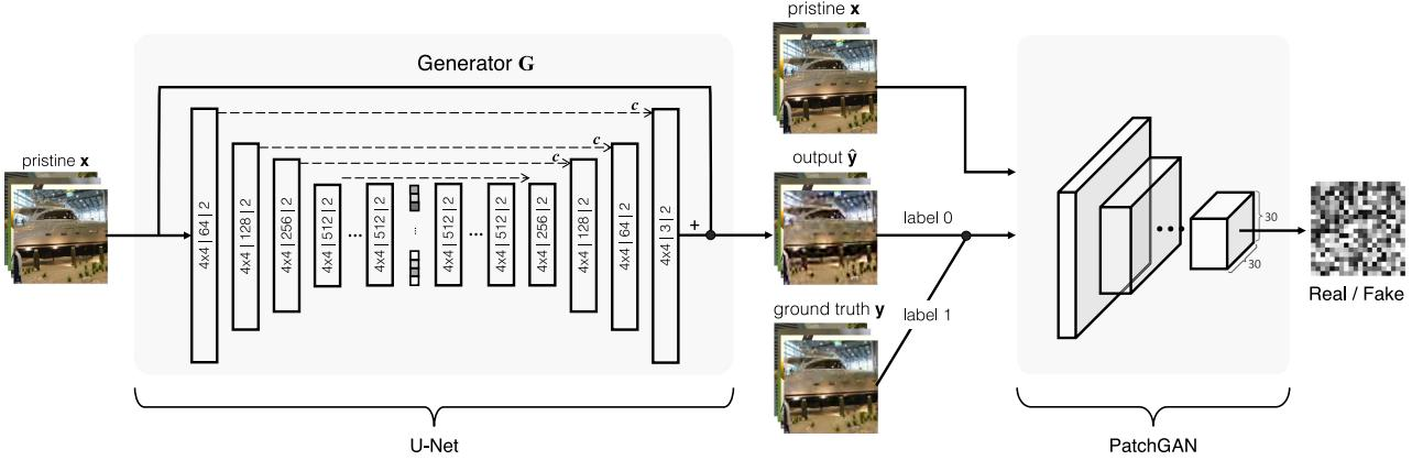
Fig. 1. Schematic diagram of how the proposed GAN-based distortion generator is trained. For each block of the generator, the convolutional parameters are denoted as: kernel size (height × width) | number of filters | stride. The operation  $c$  denotes concatenation. The discriminator is identical to PatchGAN [7].
