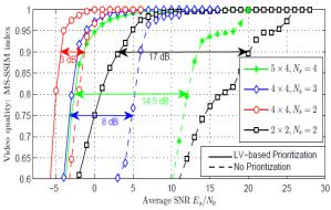
Fig. 4. Comparison of the loss visibility-based prioritization vs. non-prioritized MIMO precoding.
