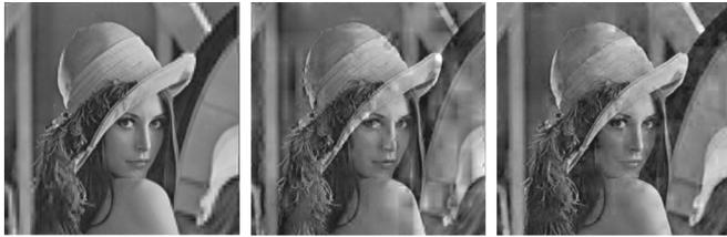
Fig. 7. (a) Reconstructed image (SSIM index = 0.9863) using the stepwise power allocation. (b) Reconstructed image using the equal power allocation (SSIM index = 0.9241). (c) Reconstructed image (SSIM index = 0.9364) using the utility-based power allocation for an MS located at the cell boundary.
