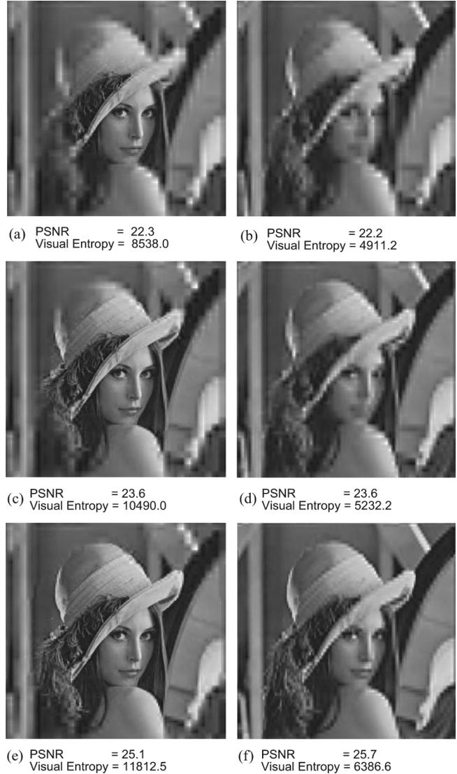
Fig. 4. Quality assessment using PSNR (in dB) versus visual entropy (in bits).
